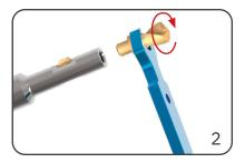
Screw tightly the drill bit with a flat wrench to the tool body.
